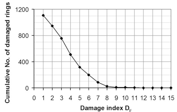
Fig. 4. Cumulated number of the fractured rings versus damage index D_F
